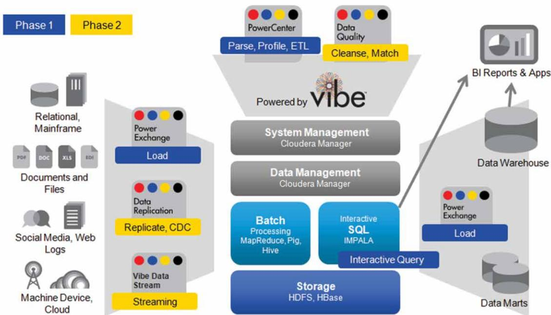
Figure 2. The Informatica/Cloudera data warehouse optimization architecture.
